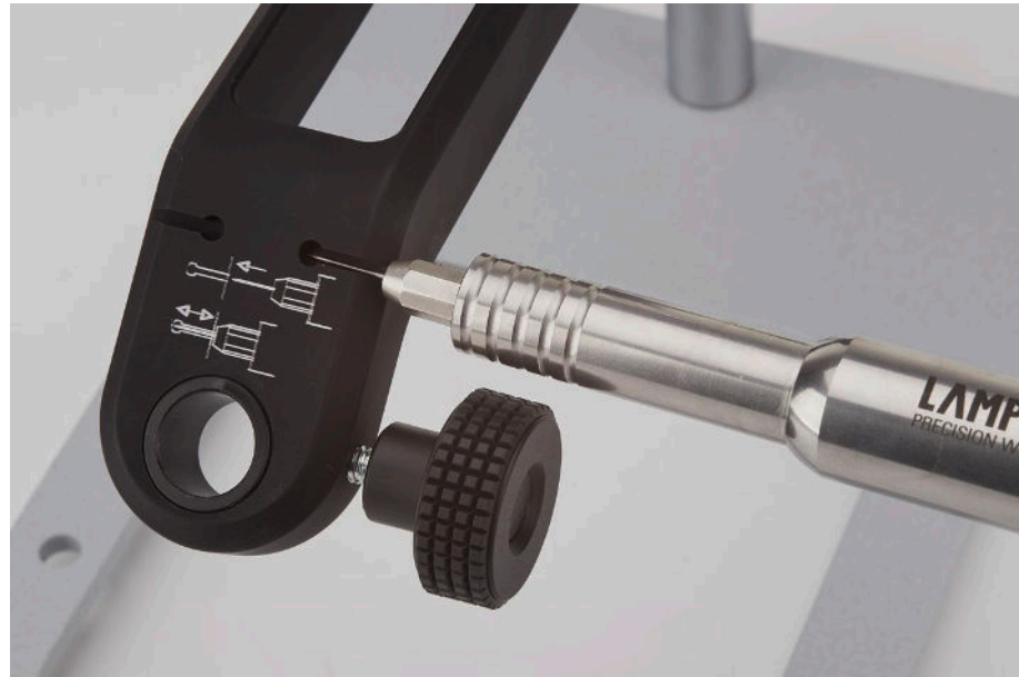
Fig. 5.2 Adjusting electrode length with handpiece holding arm
